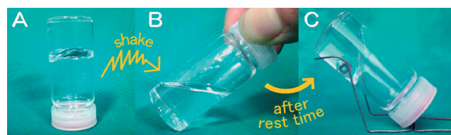
Figure 2. Photographs of decane containing 1 (30 g L -1 ). (A) Gel formed from hot solution on cooling process, (B) low-viscosity fluid formed by vigorous hand-shaking, and (C) gel reformed after left standing for a few minutes.
